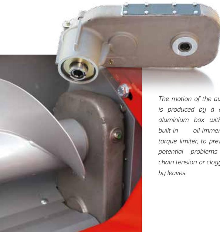
*The motion of the auger is produced by a cast aluminium box with a built-in oil-immersed torque limiter, to prevent potential problems of chain tension or clogging by leaves.*
