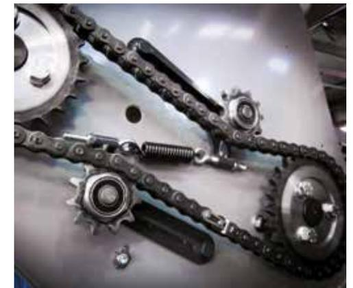
*The chain is always correctly tensioned thanks to the new active-recovery device.*
