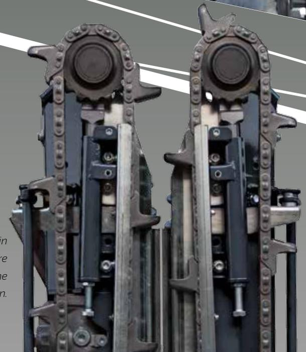
*With the new chain tensioner, bearings are protected with lifetime lubrication.*
