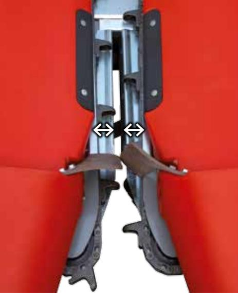
*The synchronised and simultaneous movement of the deck plates is yet another unprecedented and exclusive feature of the new DIAMANT header. In fact, both the plates move, and they do so at the same time and perfectly in sync.*
