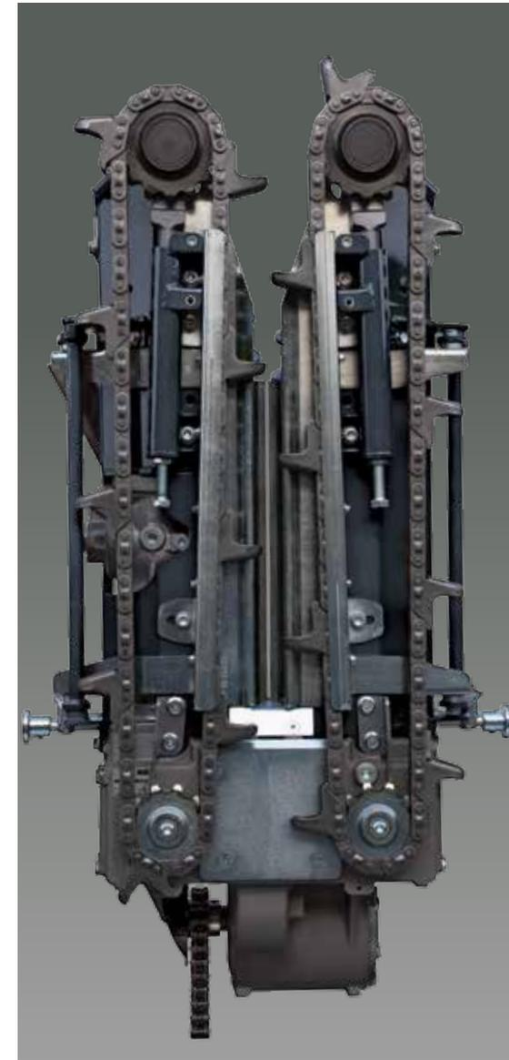
*The new fast two-blade stalk chopper is even more efficient, with minimal residue on the stalk. It can be disabled, in which case the rotor is locked.*
