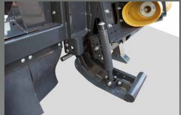
The stalk crushers (optional) protect tyres from stubble damage.
